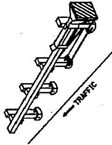
Standard Treatment - Direct Applied Sheeting Traffic Barrier Terminal Type 1 (Standard)
