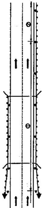
① Spacing 80 ft. (24 m) max. for first 400 ft. (122 m) or curve spacing shown in Standard 635001, whichever is less (min. 4 reflectors regardless of length).
