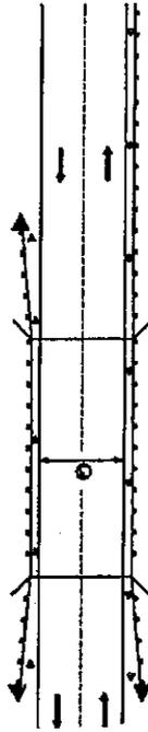
③ Bidirectional silver/silver should be used in lieu of monodirectional silver on both sides of two-lane bridges where the bridge pavement is less than 24 (610) wider than the pavement approaching the bridge.
