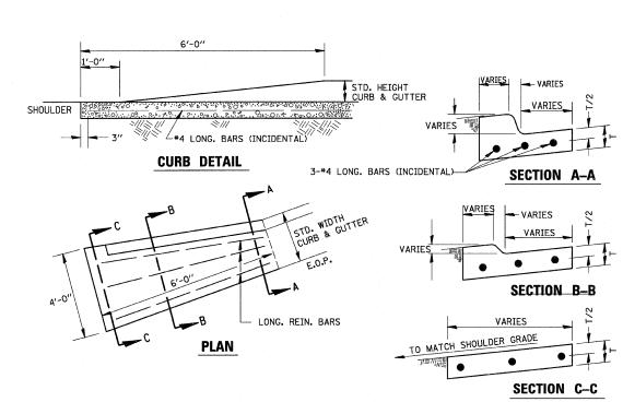
CLASS SI CONCRETE SHALL BE USED THROUGHOUT. OUTLET SHALL BE TIED TO CURB AND GUTTER AT CONTRACTION JOINTS AS SHOWN. COST TO BE INCLUDED IN THE UNIT PRICE PER CU. YD. FOR
