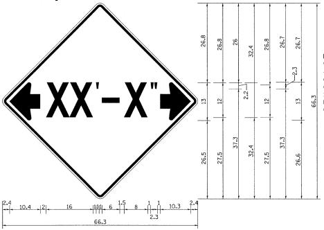
W12-2 - Horizontal Clearance Sian 48.0" across sides, 1.9" Radius, 0.8" Border, 0.5" Indent, Black on Orange; Standard Arrow Custom 10.4" X 8.1" 180° Black 11 Inch D Series Lettering; Standard Arrow Custom 10.4" X 8.1" 0°
