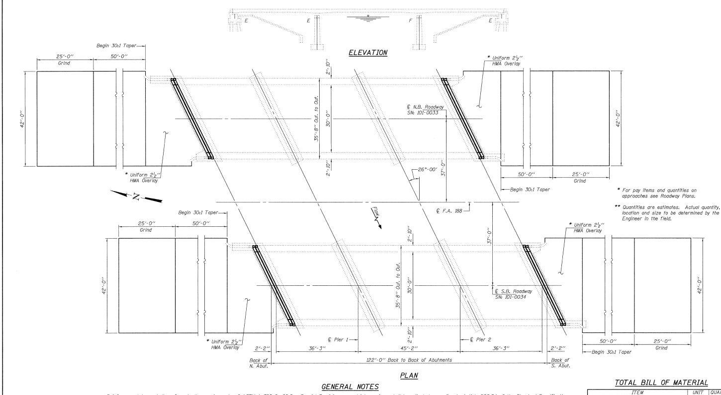
Reinforcement bars shall conform to the requirements of ASTM A 706 Gr 60.See Special Provisions. Reinforcement bars designated (E) shall be epoxy coated.
