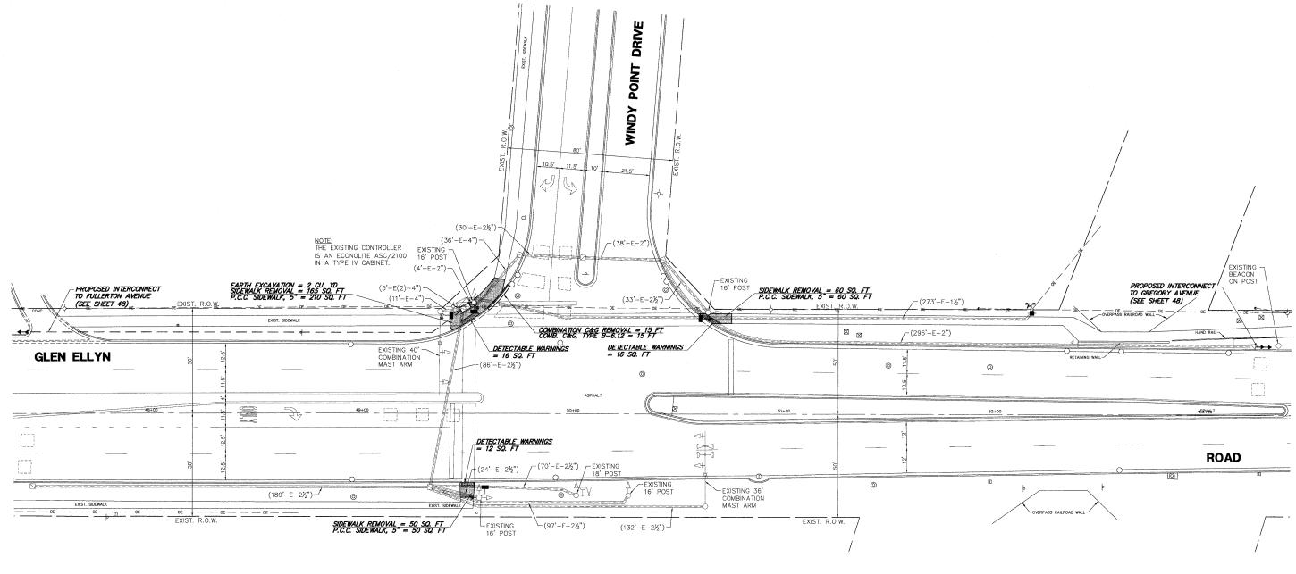
THE TRAFFIC SIGNAL CONTROL EQUIPMENT FOR THIS PROJECT SHALL BE "ECONOLITE" TO MATCH THE EXISTING ADJACENT SYSTEM. THE FOLLOWING ITEMS SHALL BE REMOVED BY THE CONTRACTOR AND SHALL BE DISPOSED OF BY THEM OUTSIDE THE RICHT-OF-WAY AT THEIR EXPENSE. THE SALVAGE VALUE OF THE REMOVED EQUIPMENT SHALL BE REFLECTED IN THE CONTRACT BID PRICE.
