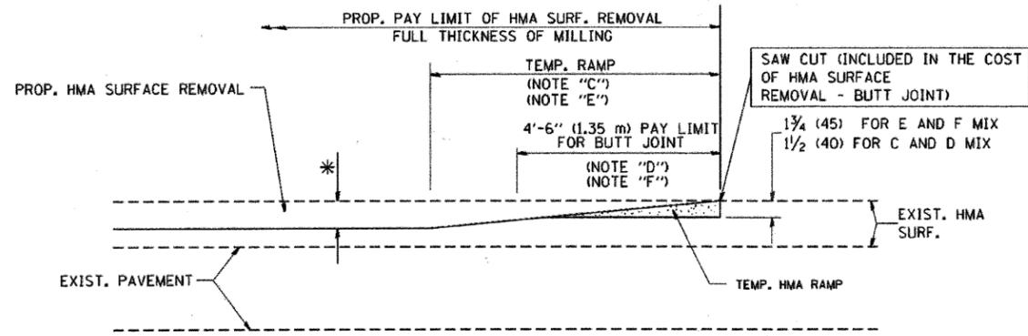
HMA CONSTRUCTED TEMPORARY RAMP
