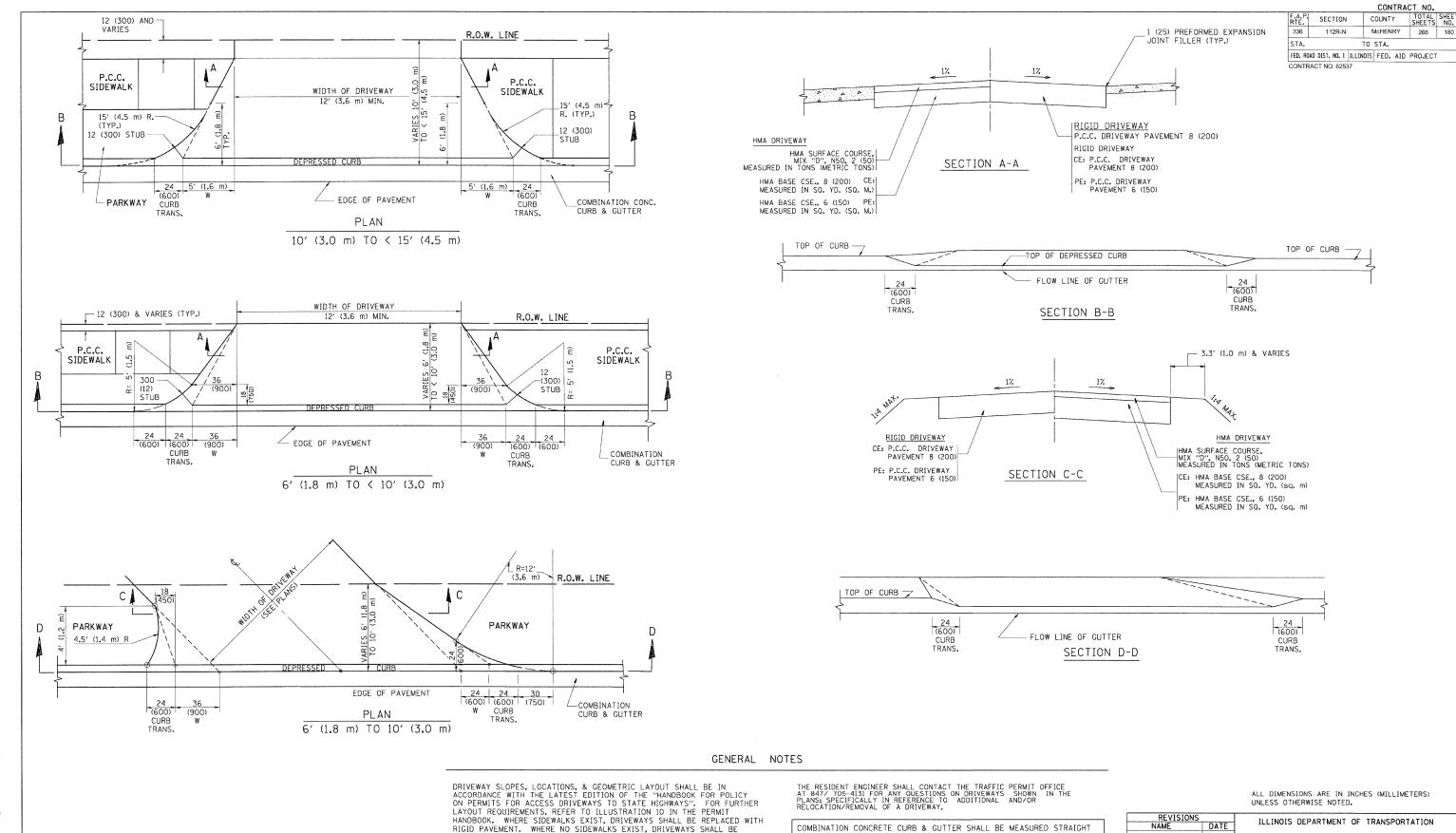
HANDBOOK. WHERE SIDEWALKS EXIST, DRIVEWAYS SHALL BE REPLACED WITH RIGID PAVEMENT. WHERE NO SIDEWALKS EXIST, DRIVEWAYS SHALL BE REPLACED IN KIND. SIDEWALK CROSS SLOPE THRU DRIVEWAY AREA TO BE A MAXIMUM OF 1:50.
