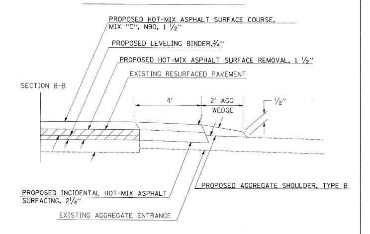
PREPARATION OF EXISTING SURFACE AND ANY EXCAVATION FOR ENTRANCES SHALL BE IN ACCORDANCE WITH ARTICLE 406.09 OF THE STANDARD SPECIFICATIONS.
