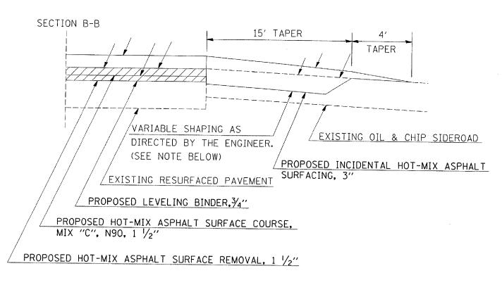
VARIABLE SHAPING IS INCLUDED IN THE COST OF INCIDENTAL HOT-MIX ASPHALT SURFACING.
