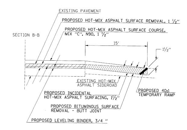
PREPARATION OF EXISTING SURFACE AND ANY EXCAVATION FOR ENTRANCES SHALL BE IN ACCORDANCE WITH ARTICLE 406.09 OF THE STANDARD SPECIFICATIONS.
