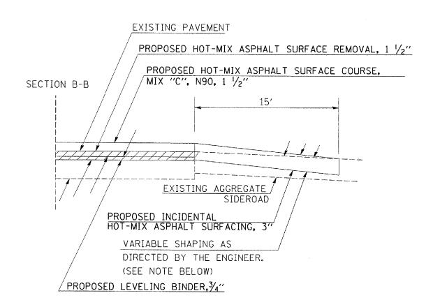
VARIABLE SHAPING IS INCLUDED IN THE COST OF INCIDENTAL BITUMINOUS SURFACING.
