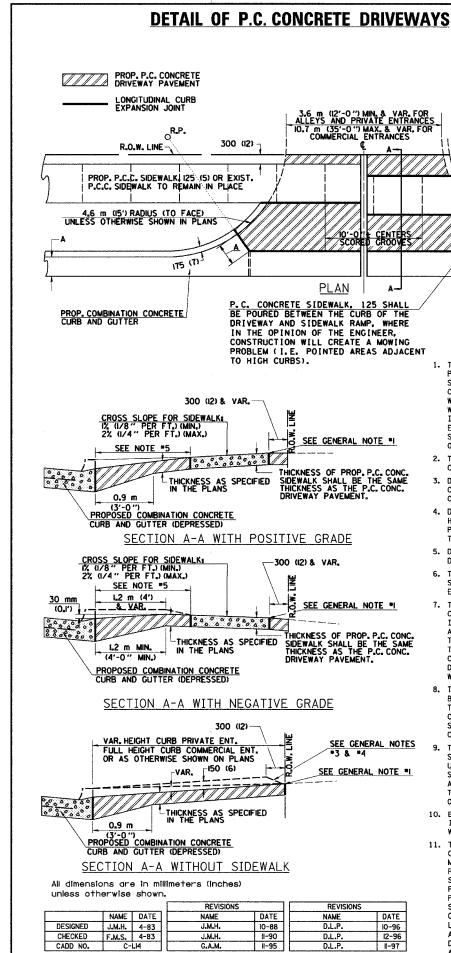
NOTE: SIDEWALK RAMPS SHALL BE CONSTRUCTED AT COMMERCIAL ENTRANCES. AT PRIVATE ENTRANCES RAMPS SHALL USUALLY BE
