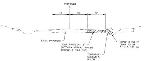
TEMPORARY PAVEMENT TYPICAL SECTION STA 124+75 TO STA 134+55
