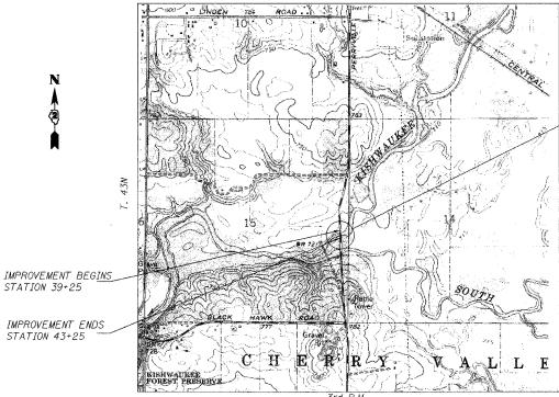
HIGHWAY CLASSIFICATION: MINOR ARTERIAL (URBAN) 2004 ADT: 4,850 1% TRUCKS DESIGN SPEED: 55 MPH POSTED SPEED: 55 MPH
