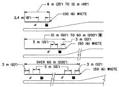
\* TURN LANES IN EXCESS OF 120 m (400°) IN LENGTH MAY HAVE AN ADDITIONAL SET OF ARROW - "ONLY" INSTALLED MIDWAY BETWEEN THE OTHER TWO SETS OF ARROW - "ONLY".
