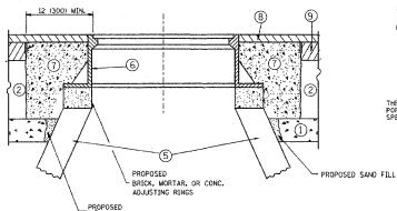
EXISTING BROKEN FRAMES AND LIDS SHALL BE REMOVED AND DISPOSED OF BY THE CONTRACTOR AND SHALL BE REPLACED AS DIRECTED BY THE ENCINEER. REPLACEMENT FRAMES AND LIDS WILL BE PAID FOR IN ACCORDANCE WITH ARTICLE 109,04 OF THE STANDARD SPECIFICATIONS UNLESS A SEPARATE PAY ITEM HAS BEEN PROVIDED.
