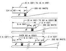
\* TURN LANES IN EXCESS OF 120 m (400") IN LENGTH MAY HAVE AN ADDITIONAL SET OF ARROW - "ONLY" INSTALLED MIDWAY BETWEEN THE OTHER TWO SETS OF ARROW - "ONLY".
