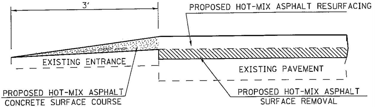
FEATHEREDGE DETAIL FOR OIL AND CHIP, HOT-MIX ASPHALT, AND CONCRETE ENTRANCES (PAID FOR AS HOT-MIX SURFACE COURSE)
