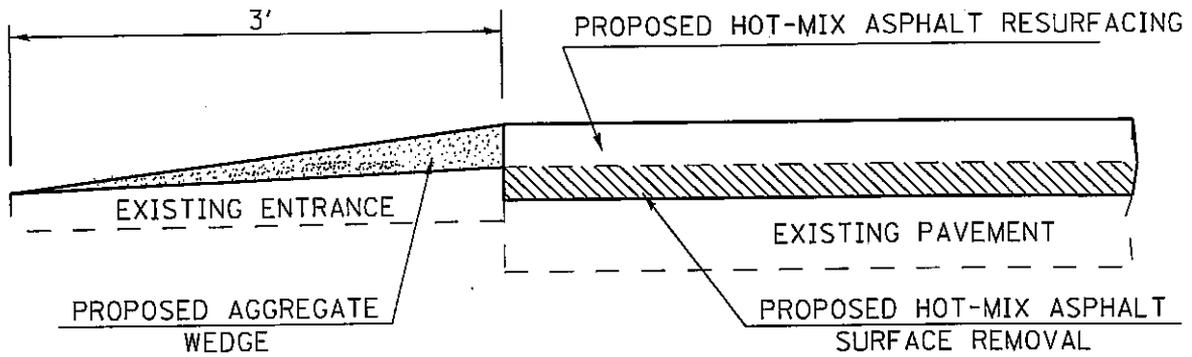
FEATHEREDGE DETAIL FOR AGGREGATE ENTRANCES (PAID FOR AS AGGREGATE SHOULDER, TYPE B)
