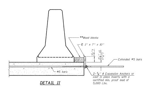
\*\* Wood blocks may be omitted when required to provide minimum stage traffic lane width. When the wood blocks are omitted, the concrete barrier shall be in direct contact with the steel retainer plate.
