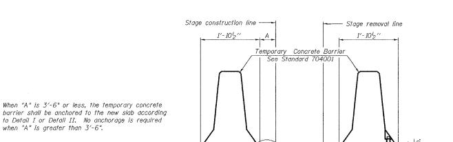
Drill 14" \$ Holes in existing See Detail I slab for 1"  $\phi$  x 11" dowel bars. Traffic side only. Cost included
