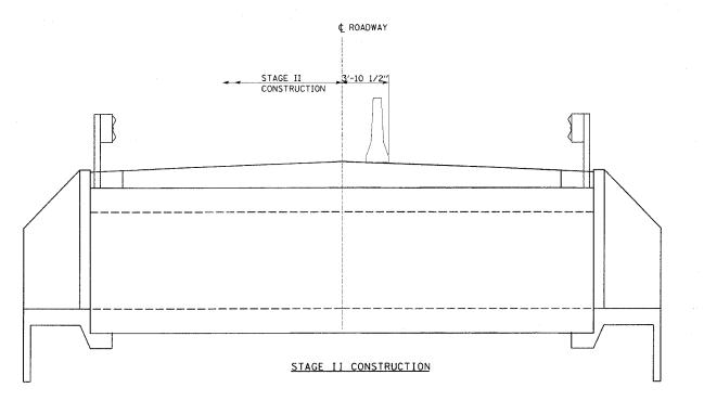
NOTES: ALL STAGING CROSS SECTIONS ARE LOOKING NORTHWEST. HATCHED AREA INDICATES REMOVAL OF EXISTING STRUCTURES. FOR QUANTITY OF TEMPORARY CONCRETE BARRIER, SEE ROADWAY PLANS.
