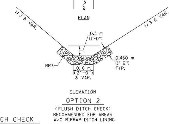
**STONE DUMPED RIPRAP DITCH CHECK**
