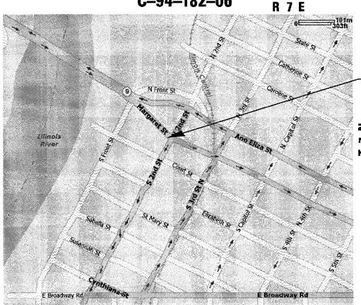
DESCRIPTION OF WORK: THIS PROJECT CONSISTS OF WIDENING THE RADIUS OF THE RIGHT TURN LANE ON MARGARET STREET BY REMOVING AND REPLACING A PORTION OF IT WITH NEW CONCRETE PAVEMENT.
