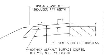
t = SEE TYPICAL SECTIONS FOR THICKNESS
