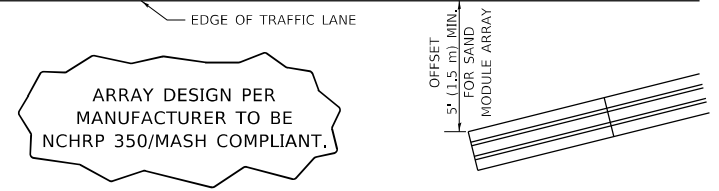
DETAIL "A" IMPACT ATTENUATOR, TEMPORARY (SEE NOTE 5)
