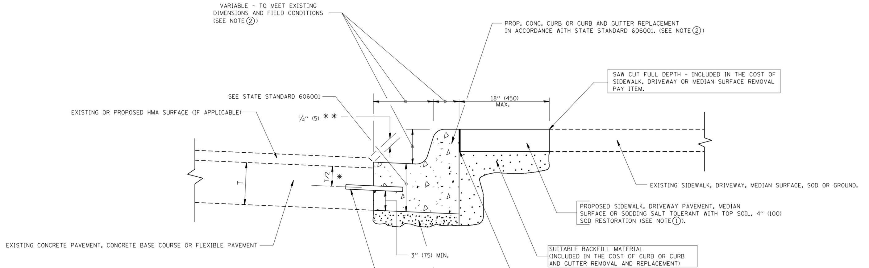
\* 3" (75) MINIMUM FROM TOP AND BOTTOM OF THE CONCRETE PAVEMENT OR BASE COURSE.
