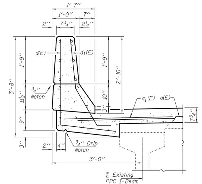
**SECTION THRU PARAPET (DECK)**
