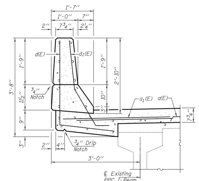
**SECTION THRU PARAPET (DECK)**
