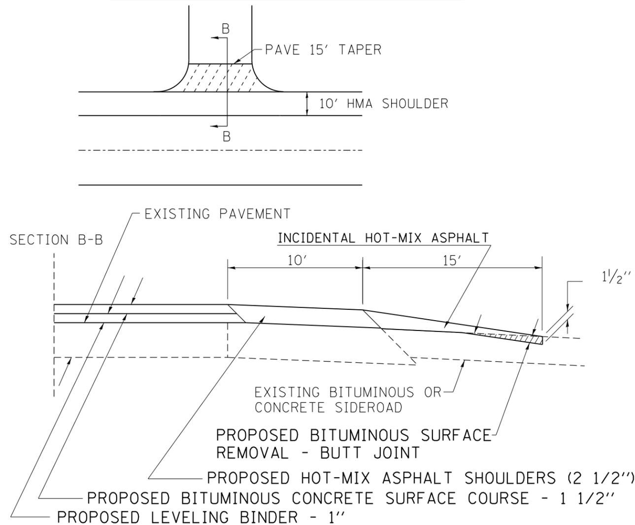
IF EXISTING BASE COURSE IS INADEQUATE, AS DETERMINED BY THE ENGINEER, THE SIDEROADS SHALL BE CORED OUT AND AGGREGATE BASE COURSE, TYPE B SHALL BE PLACED FOR BASE. THE COST OF CORING OUT THE SIDEROAD SHALL BE INCLUDED IN THE COST OF THE AGGREGATE BASE COURSE. IF EXISTING BASE COURSE IS DETERMINED TO BE ADEQUATE, THE AGGREGATE BASE COURSE SHALL BE DELETED AND THE PREPARATION OF THE BASE SHALL BE CONSTRUCTED ACCORDING TO ARTICLE 406.09.
