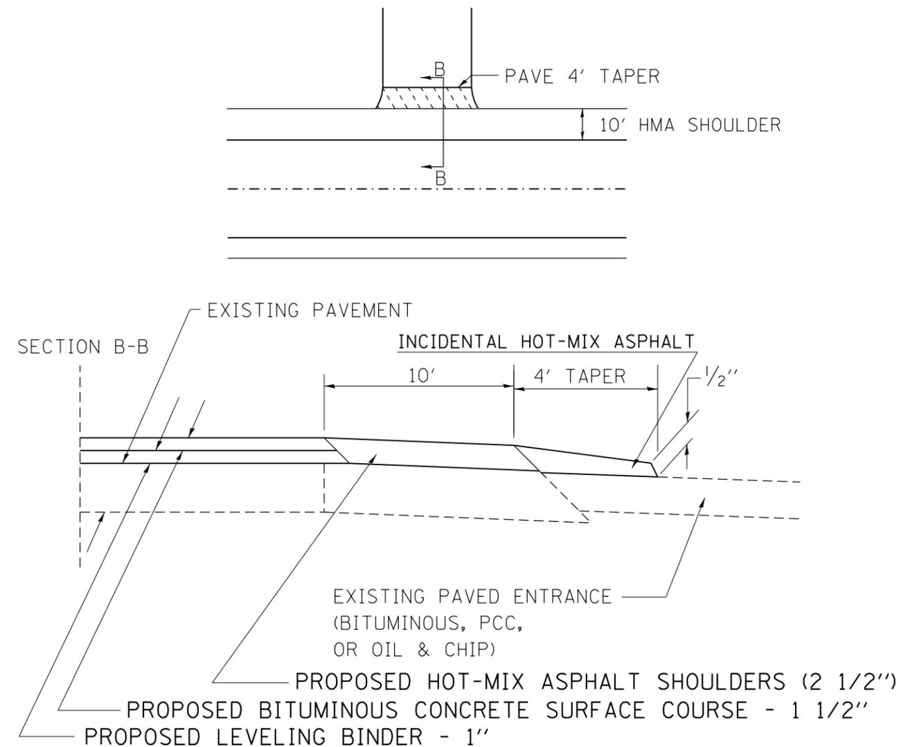
PREPARATION OF EXISTING SURFACE AND ANY EXCAVATION FOR ENTRANCES SHALL BE IN ACCORDANCE WITH ARTICLE 406.09 OF THE STANDARD OF SPECIFICATIONS.
