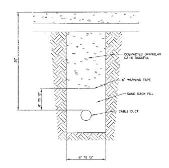
TRENCH & BACKFILL -CONCRETE AND ASHPALT AREA IF TRENCH IS USED N.T.S.
