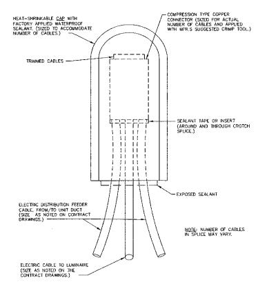
ELECTRICAL CABLE SPLICE DETAIL N.T.S.
