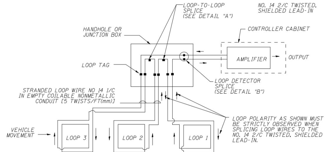
**DETECTOR LOOP WIRING SCHEMATIC**
