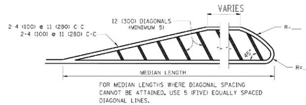
FOR MEDIAN LENGTHS WHERE DIAGONAL SPACING CANNOT BE ATTAINED, USE 5 (FIVE) EQUALLY SPACED DIAGONAL LINES.
