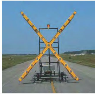
LIGHTED RUNWAY CLOSURE MARKER NOT TO SCALE
