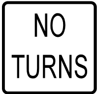
R3-3 36" x 36" D FURNISH & INSTALL FIVE (5) EACH SIGN DETAIL OF SIGN PANEL - TYPE 1 (NOT TO SCALE)
