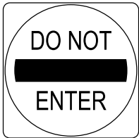
R5-1 36" x 36" K FURNISH & INSTALL ONE (1) EACH SIGN DETAIL OF SIGN PANEL - TYPE 1 (NOT TO SCALE)
