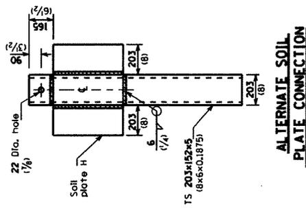
**ALTERNATE SOIL PLATE CONNECTION**
