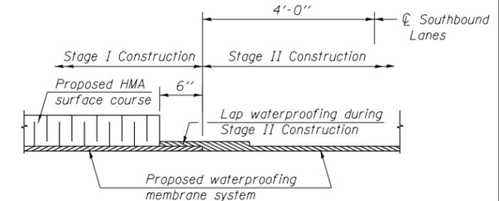
**WATERPROOFING TREATMENT AT STAGE CONSTRUCTION**
