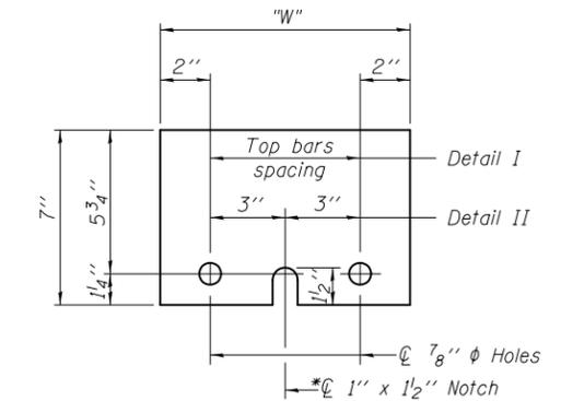
**STEEL RETAINER  $\bar{L}$  1" x 7" x "W"**
