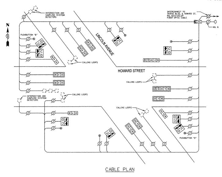
PUSHBUTTON "B" SHALL PLACE A CALL TO PHASES 4 & 6 PUSHBUTTON "D" SHALL PLACE A CALL TO PHASES 2 & 8
