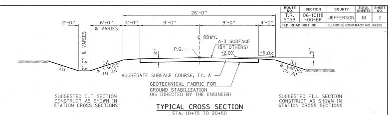
TRANSITION FROM THE PROPOSED ROADWAY TO THE EXISTING ROADWAY IS TO BE CONSTRUCTED FROM STA. 10+75 TO 11+25 AND STA. 20+00 TO 20+50. SEE SHEET 11 FOR TRANSITION AT BRIDGE.
