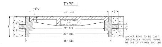
THE FRAMES MAY BE MADE OF EITHER GRAY IRON CONFORMING TO THE STANDARD SPECIFICATIONS OR DUCTILE IRON CONFORMING TO THE SPECIFICATIONS FOR DUCTILE IRON CASTING, A.S.T.M. DESIGNATION: A536, GRADE 60-45-10.
