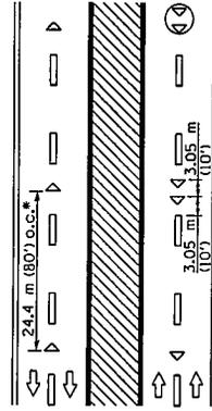
\* Reduce to 12.2 m (40') o.c. on curves where advisory speeds are 15 km/h (10 mph) lower than posted speeds.
