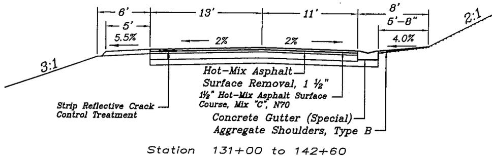
NOTE: FINAL PAVEMENT MARKINGS SHALL MATCH EXISTING PAVEMENT MARKINGS
