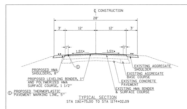
¢ CONSTRUCTION 28' 3′ 12' 3′ 12' 1.5%\* 1.5%\* EXISTING CONCRETE GUTTER PROPOSED THERMOPLASTIC EXISTING AGGREGATE PAVEMENT MARKING LINE, 5" BASE COURSE PROPOSED POLYMERIZED HMA EXISTING CONCRETE SURFACE COURSE, 2" PAVEMENT PROPOSED HMA SURFACE/ REMOVAL, 2" EXISTING HMA BINDER & SURFACE COURSE
