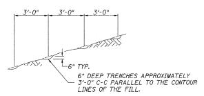
NOTE: ALL SLOPES 3:1 OR STEEPER AND GREATER THAN 5' IN HEIGHT SHALL BE CONTOUR PLOWED AS SHOWN IN DETAIL, COST SHALL BE INCLUDED WITH SEEDING, CLASS 2 (SPECIAL).
