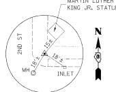
CONTROL POINT 50 DRILL HOLE IN CONC SIDEWALK 31+10.48, 33.98'LT N 34.000, E 1010.000
