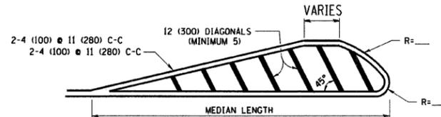
FOR MEDIAN LENGTHS WHERE DIAGONAL SPACING CANNOT BE ATTAINED, USE 5 (FIVE) EQUALLY SPACED DIAGONAL LINES.
