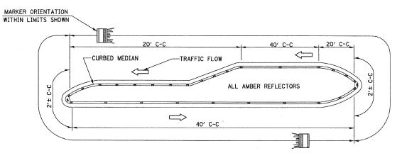
NOTES 1. PRISMATIC REFLECTORS SHALL BE MONO-DIRECTIONAL AND POSITIONED SO THAT THE REFLECTIVE FACE IS FACING THE APPROACHING TRAFFIC.
