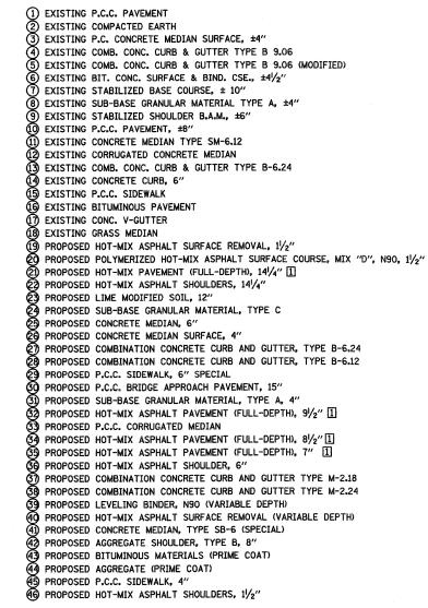
NOTE: THE TOP 2" OF FULL DEPTH HOT-MIX ASPHALT SHALL MEET THE REQUIREMENTS OF "POLYMERIZED HOT-MIX ASPHALT SURFACE COURSE, MIXTURE D, N90." THE REMAINDER SHALL MEET THE REQUIREMENTS OF "HOT-MIX ASPHALT BINDER COURSE, IL-19.0, N90."
