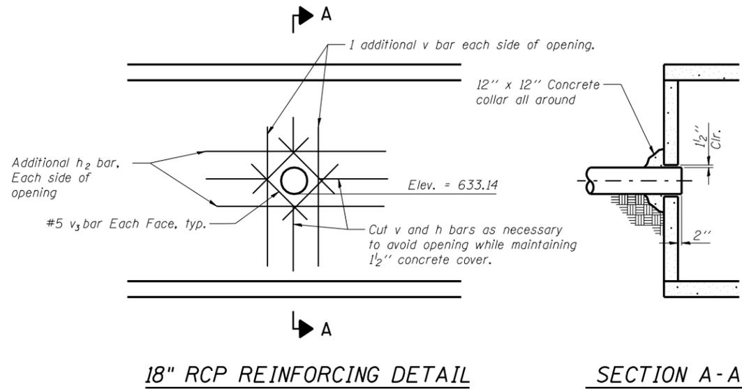
Note: At the Contractor's option delete the concrete collar and cast the wall around the pipe.
