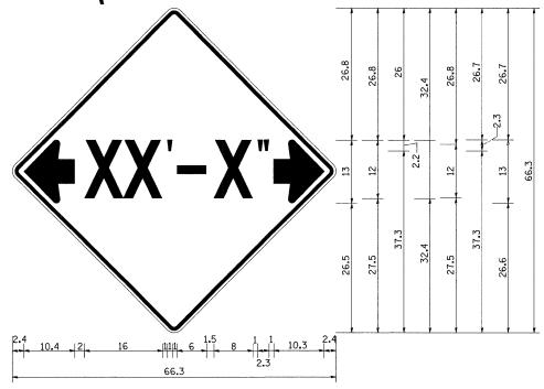
W12-2 - Horizontal Clearance Sign 48.0" across sides, 1.9" Radius, 0.8" Border, 0.5" Indent, Black on Orange; Standard Arrow Custom 10.4" X 8.1" 180° Black 11 Inch D Series Lettering; Standard Arrow Custom 10.4" X 8.1" 0°
