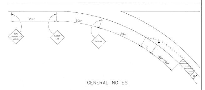
CONES AT 8 m (25')CENTERS FOR 105 m (350'). ADDITIONAL CONES MAY BE PLACED AT 15 m (50') CENTERS. WHEN DRUMS OR BARRICADES ARE USED. THE INTERVAL DEVICES MAY BE DOUBLED.
