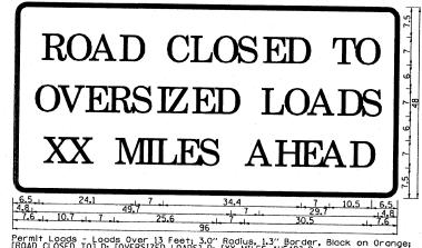
Permit Loads - Loads Over 13 Feet; 3.0" Radius, 1.3" Border, Black on Orange; [ROAD CLOSED TO] D; [OVERSIZED LOADS] D; [XX MILES AHEAD] D; Table of letter and object lefts.
