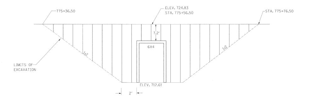
TEMPORARY SOIL RETENTION SYSTEM STAGE I
