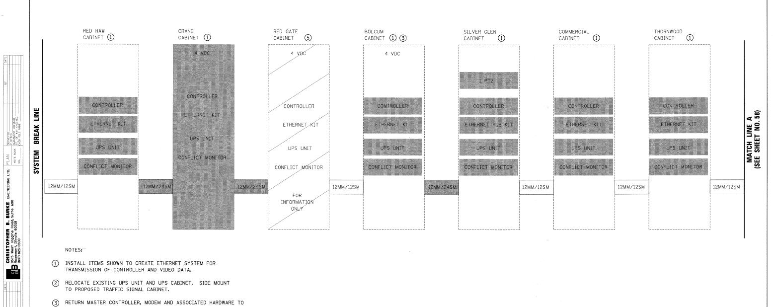
4 REPLACE VIDEO PROCESSING UNIT TO COMMUNICATE OVER ETHERNET.
