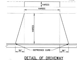
THIS TYPICAL DRIVE LAYOUT IS FOR BOTH CONCRETE AND ASPHALT DRIVES
