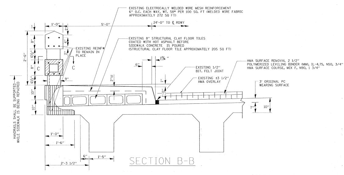
\* EXISTING REINFORCEMENT BARS EXTENDING INTO THE REMOVAL AREA SHALL BE CLEANED, STRAIGHTENED AND INCORPORATED INTO THE NEW CONSTRUCTION. ANY REINFORCEMENT BARS THAT ARE DAMAGED DURING CONCRETE REMOVAL SHALL BE REPLACED WITH AN APPROVED BAR SPLICER OR ANCHORAGE SYSTEM. COST INCLUDED WITH CONCRETE REMOVAL.
